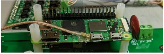
□ **RPi/FEZ only**: The standoff between the relays will need a nut installed as a spacer as shown.
