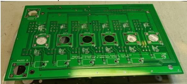
NOTE that the ground side of the components may be difficult to solder. The ground plane is a pretty good heat sink. Make sure your soldering iron and tip are of adequate size and the tip is well wetted.
