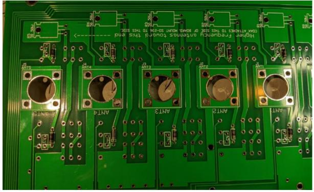
☐ Solder the diodes as shown. Clip the leads flush.
